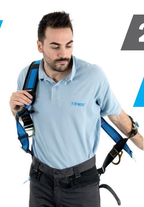
Put harness on like a jacket. Dorsal D-ring should be placed between shoulder blades.
